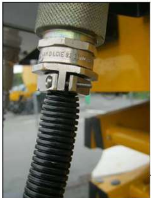
The corrugated hose has to be hold by the plug adaptor as showed in the picture
